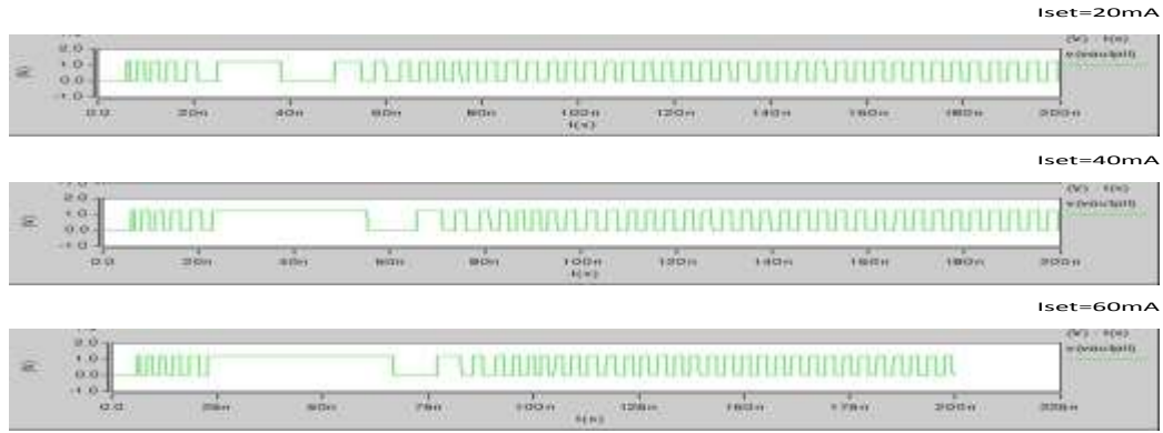
Fig: Simulation result for Voutpll signal with SE strike of 20mA, 40mA & 60mA at 20nsec
